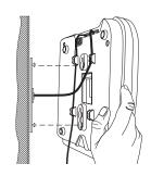
4. Plug the AC Adapter into a standard 120V AC wall outlet.
